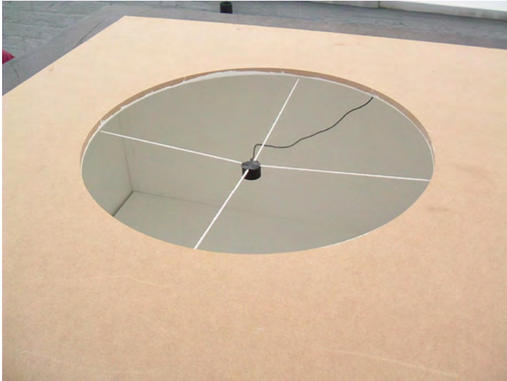
Figure 3 The aperture plate on top of the integrating box. The back of the photocell is visible through the aperture. The underneath of the plate is painted matt white.
